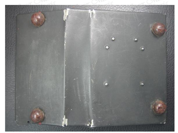
A 25 x 18cm aluminum access panel from Junkers 88, possibly from the cockpit. Panel is painted the standard green/grey, with four round bakelite spring loaded catches. To the unpainted reverse are the catches themselves and the following is engraved:
